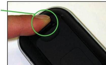
Observe the + and - polarity indications inside the battery compartment.
