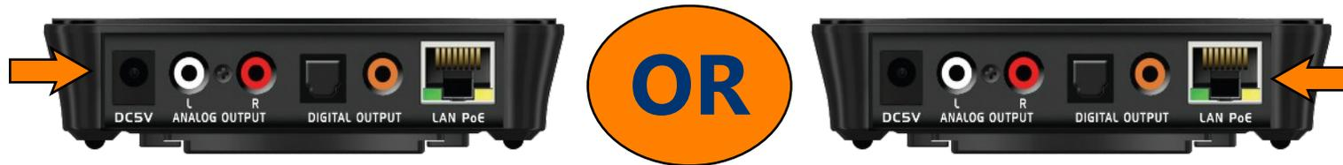
2. Connect an Ethernet cable from the LAN 10/100 port to an MFS-8/MFSPOE-8
