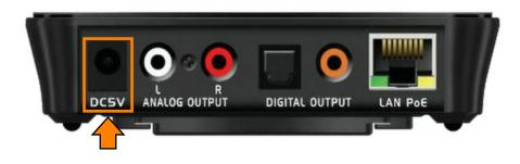
**Analog Output:** Standard RCA out (analog) connector.
