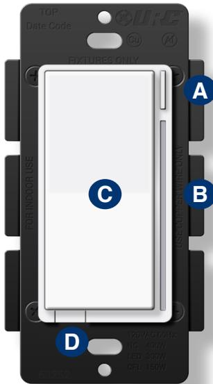
**A. Config Button:** This button is used to enter the configuration menu on your dimmer. When you hold it down for 10-15 seconds, the **LED Bar (B)** will light up **Yellow** to indicate you are in config mode. It can also be used to trigger a favorite scene. After setting up the scene, tap the button one time to trigger it.
